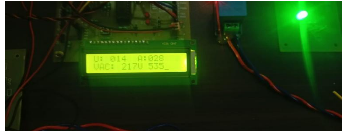
FIG. 2: LCD DISPLAY SHOWING REAL-TIME VOLTAGE AND CURRENT MEASUREMENTS.
