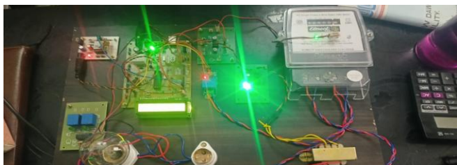
FIG. 1: EXPERIMENTAL SETUP OF IOT-BASED ENERGY METER SYSTEM.
