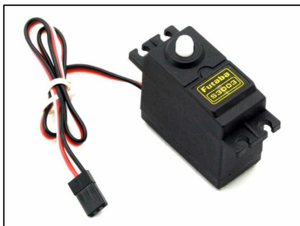
FIG. 9 SERVO MOTOR TO OPERATE DUSTBIN DOOR
